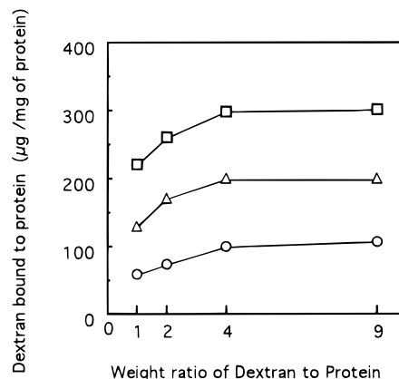
Figure 1. Effect of dextran on glycosylation of Mf. Mf was reacted with different amounts of dextran at 40 °C for 24 h (○), 40 °C for 48 h (△), and 50 °C for 48 h (□).
